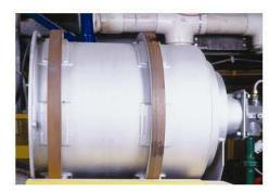
FEECO has the ability to test your material in our laboratory both in batch and pilot scale tests. The rotary batch kiln, shown here, is used to observe the behavior of material as it is heated using a programmed temperature profile. This profile is matched to that expected in a commercial kiln.
